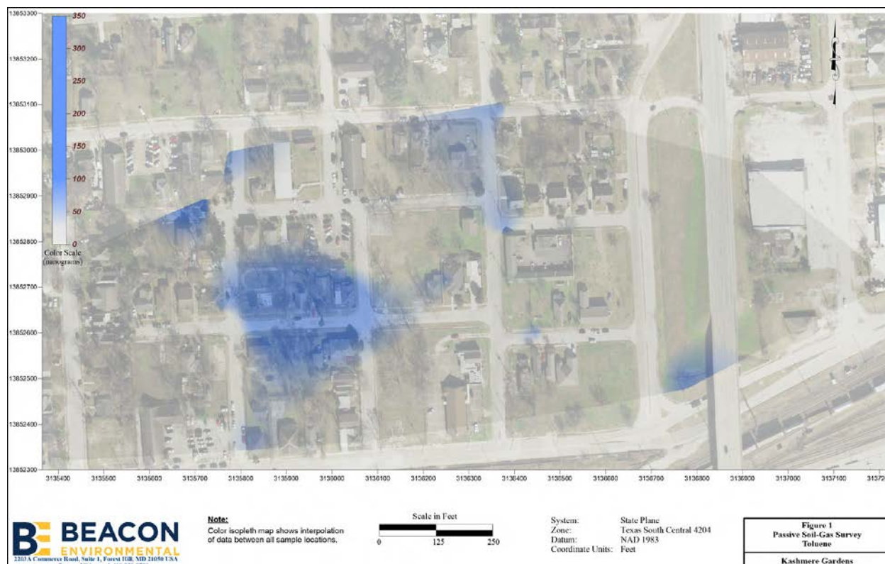
Map 2 – Isopleth Map Depicting Extent of Toluene in the Form of Vapors as a Result of November 2020 Survey
