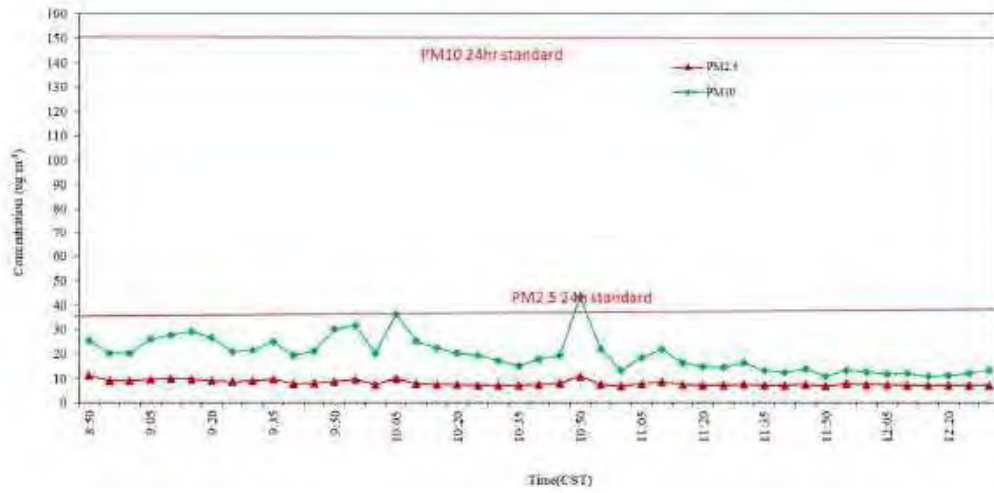
Figure 2: Time series graph of PM 10 and PM 2.5 concentrations – Lyndon B Johnson Hospital (08/31/23)
