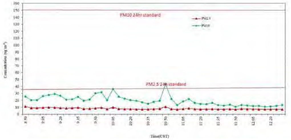
Figure 2: Time series graph of PM 10 and PM 2.5 concentrations – Lyndon B Johnson Hospital (08/31/23)
